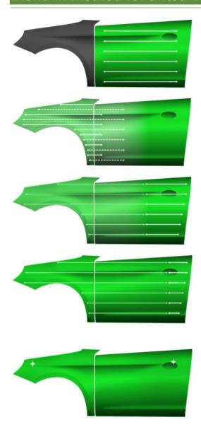
Adjacent panel: sand panel with suitable abrasive e.g. Trizact – P1000. New part / repair: sand filler (minimum P500).
